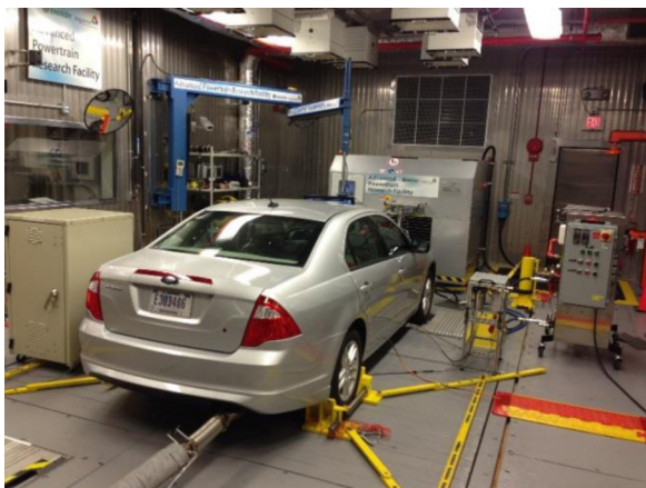
Figure 1. 2011 Ford Fusion test vehicle on APRF dynamometer for testing. Photo by Forrest Jehlik, Argonne National Laboratory
